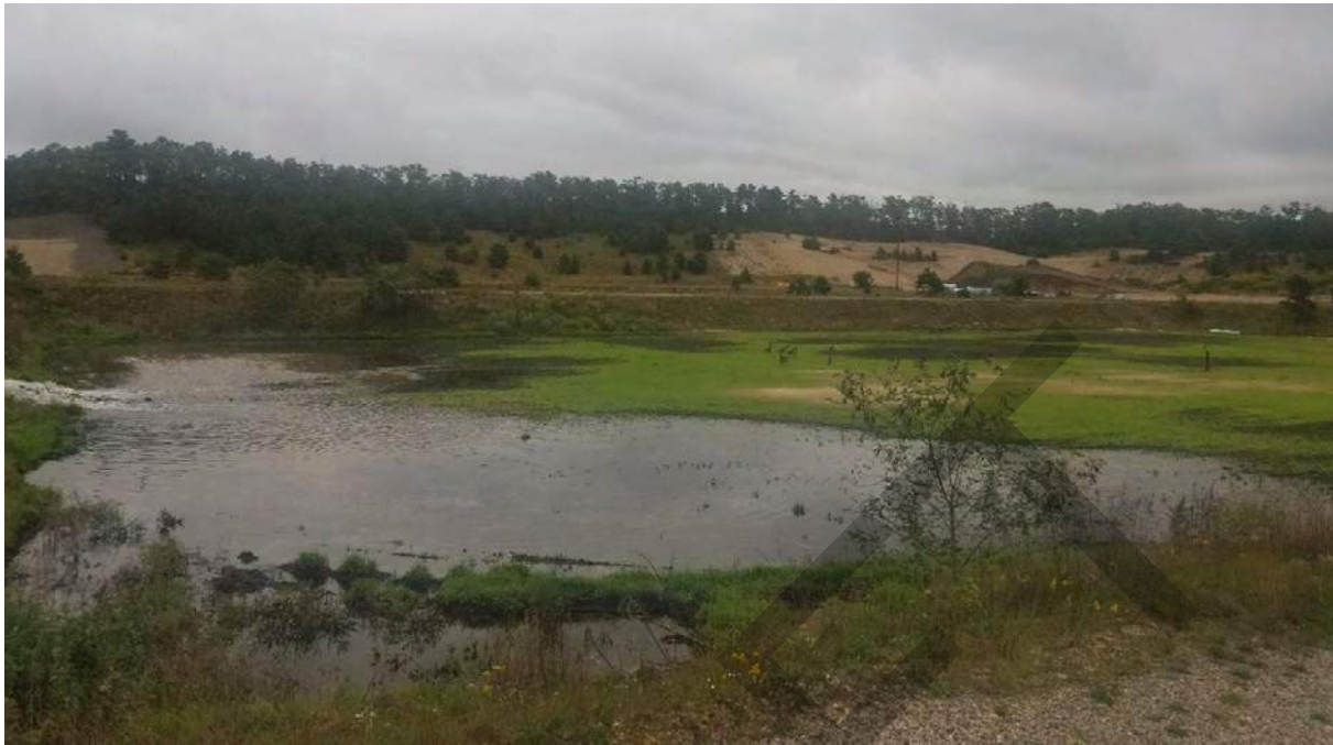
Photo 1: Bed #4 receiving treated effluent during the loading test.
